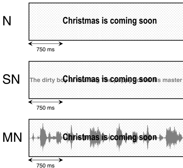
FIG. 1. A schematic illustration of the three stimulus conditions of experiment 1. The open black box represents the steady noise present in each condition. The text Christmas is coming soon represents the target speech, which starts 750 ms after the steady noise in each condition. In the SN condition (middle panel) the gray text represents the competing speech (“The dirty boy was washing the puppy licked his master”). In the MN condition (bottom panel) the gray waveform represents the modulated noise.
